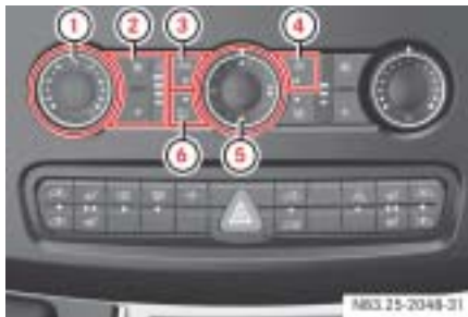
Control panel for the air-conditioning system
