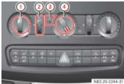
Heater control panel
