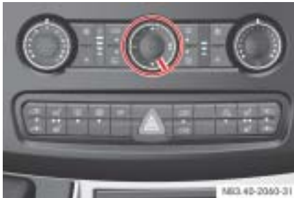
Air distribution control
